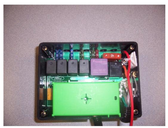
Refer to the circuit board picture below for clarification of fuse/relay locations in the Controls Pack PDB.
